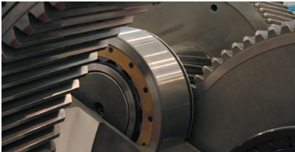
Fig. 3: Gear efficiency is determined to a large extent by the friction characteristics of the lubricating oil.
